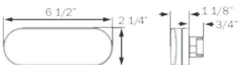
HOLE CUT-OUT: 6.85" x 2.5" (1.25" R)
