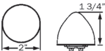
MCL21 SERIES HOLE CUT-OUT: 2.313"
