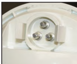
ST45RGB male pin connection detail
