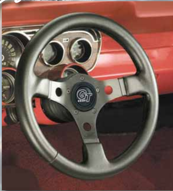
773 Formula GT Model shown with standard installation kit
