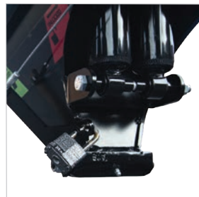
Lockable BULLDOG® coupler for added security
