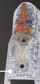
Competitor's Coupler After 336 Hours Salt Spray Testing
