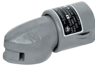
2B Style: 5,000 lbs. Gross Trailer Weight for 2" Ball
