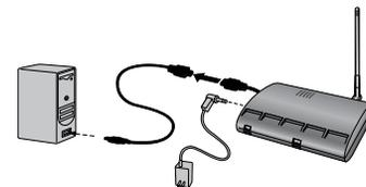
Install Weather Envoy close to your computer using the included USB cable and AC adapter.
