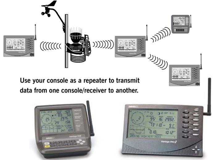
Use your console as a repeater to transmit data from one console/receiver to another.
